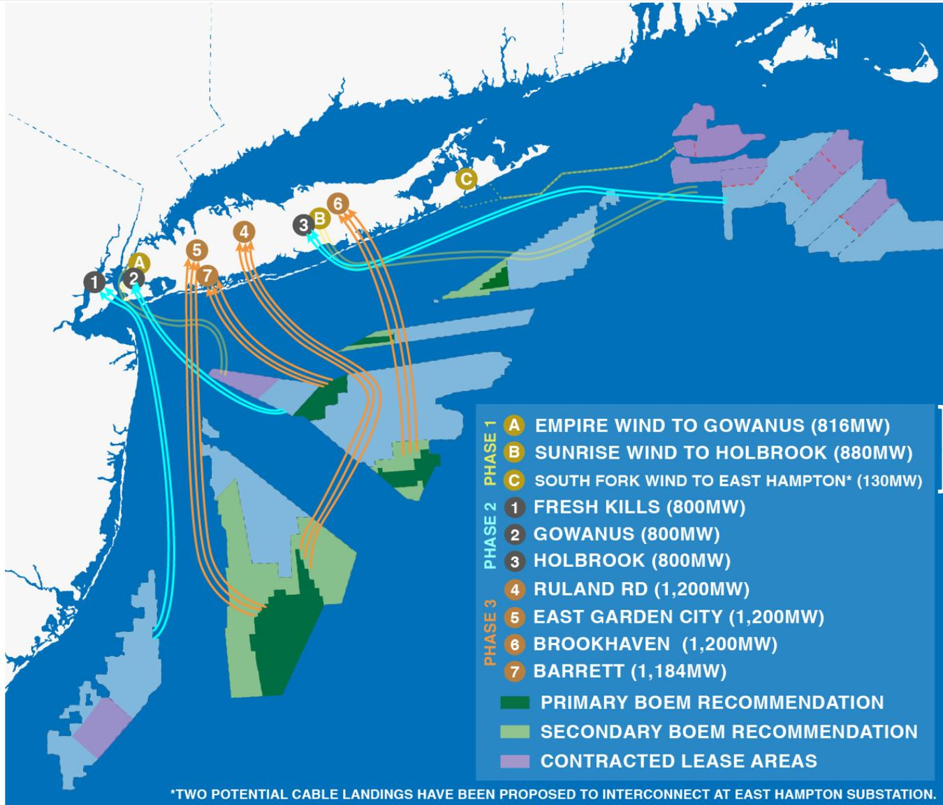
Phase 1 is already contracted using HVAC cables. In the GLL scenario, projects in Phases 2 and 3 also use HVAC lines.
