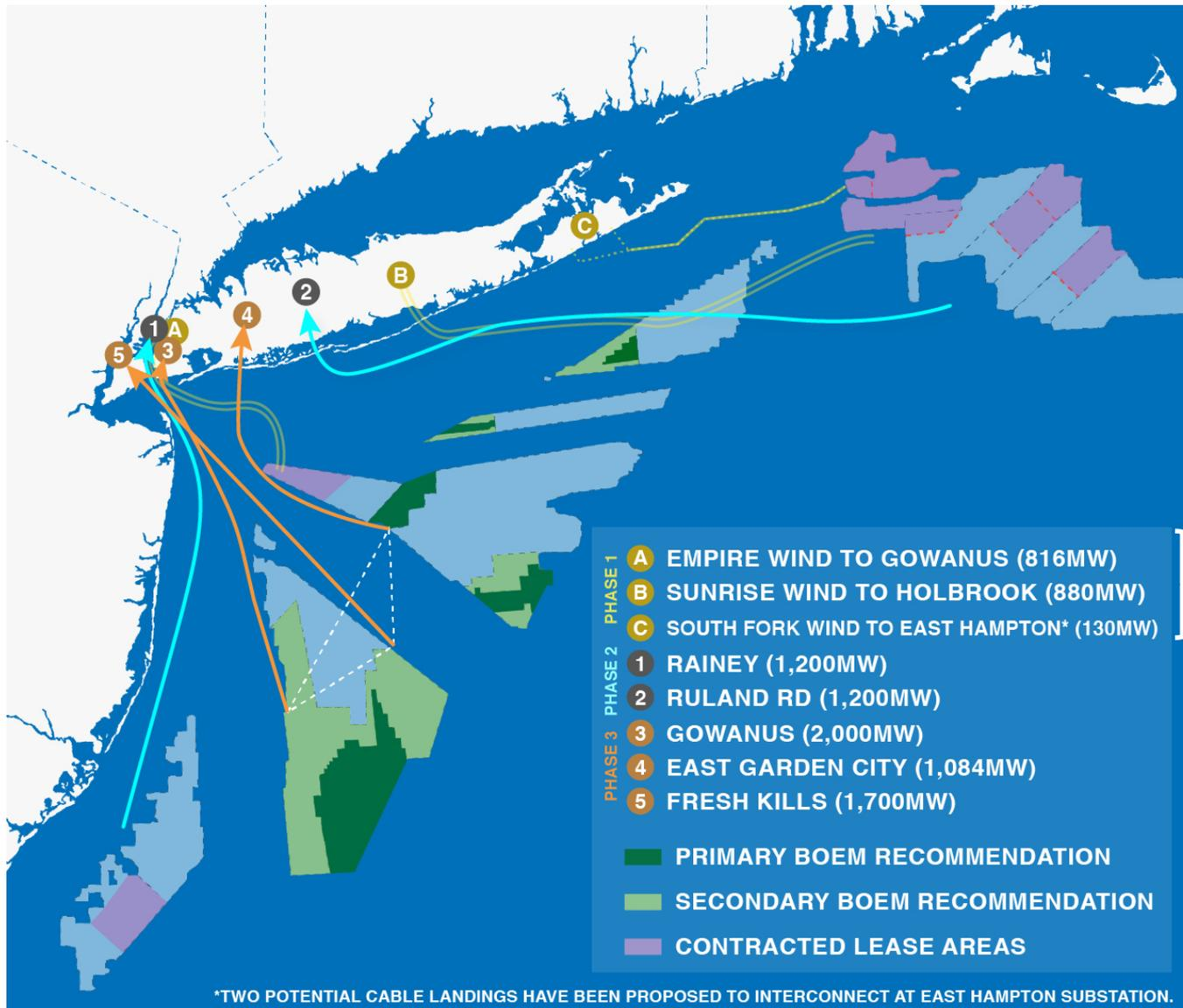
Phase 1 is already contracted using HVAC cables. Planned approach utilizes **HVDC cables** for Phases 2 and 3.
