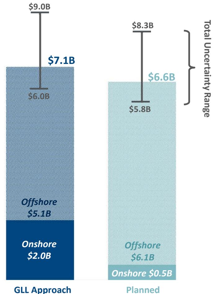
Source for cost data: Onshore upgrade cost estimates based on Pterra power flow modeling and PSC Consulting analysis of reliability transmission upgrades. See Appendix B. Does not include elective transmission upgrades. Estimate for offshore transmission equipment based on proprietary supplier information provided to Anbaric. We assumed +25%/-10 uncertainty for the offshore cost, plus the uncertainty for the onshore upgrades given by PSC.
