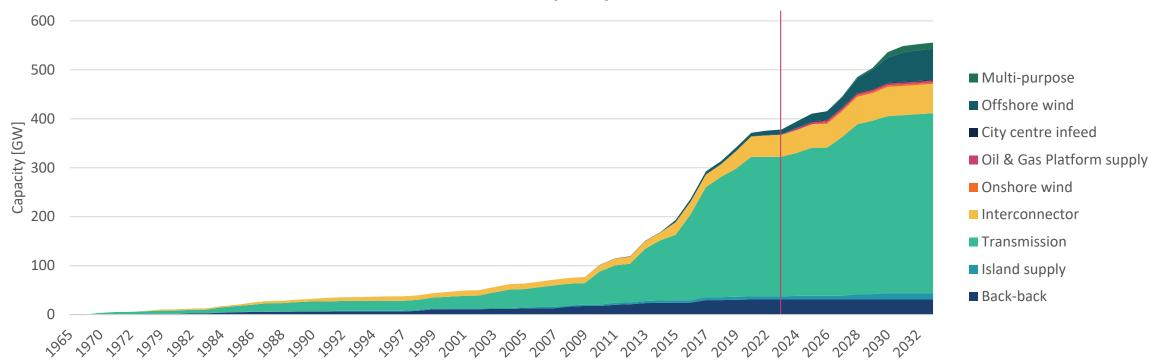
**HVDC** transmission capacity installed worldwide
